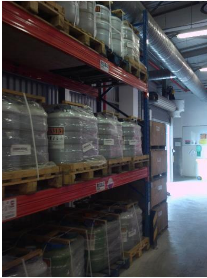
Photo 3. Storage of liquid hazardous chemicals in Room 101 (not designed for such storage)
