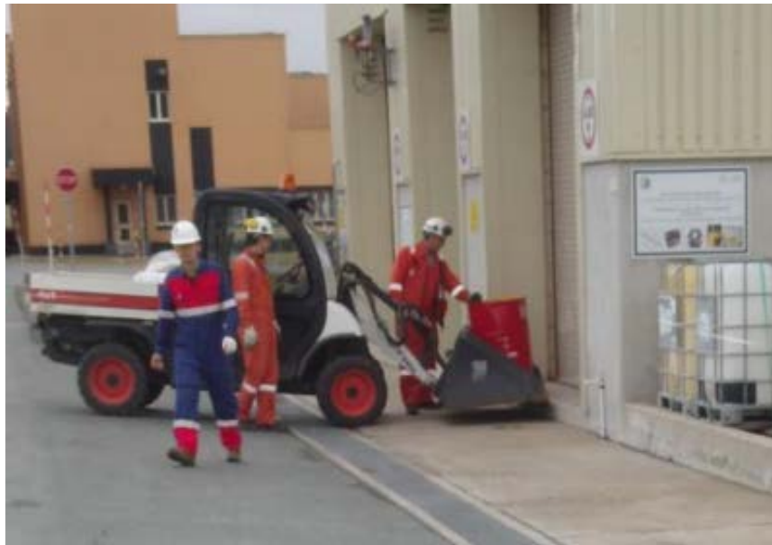
Photo 2. Waste oil drum transported by Bobcat – unsecured – outside Building 10 (over storm water drain)
