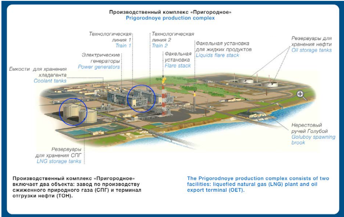
Figure 2 - Layout of Prigorodnoye Production Complex (from Sakhalin Energy website)
