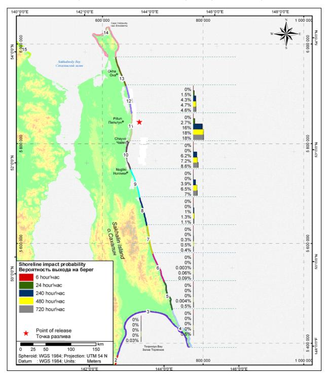
*Figure 2.4 Probability of Shoreline Impact from Piltun-A Platform (Molikpaq): Autumn* (Scenario: Volume: 96m<sup>3</sup>; Cause: Pipeline rupture, REA 2004)
