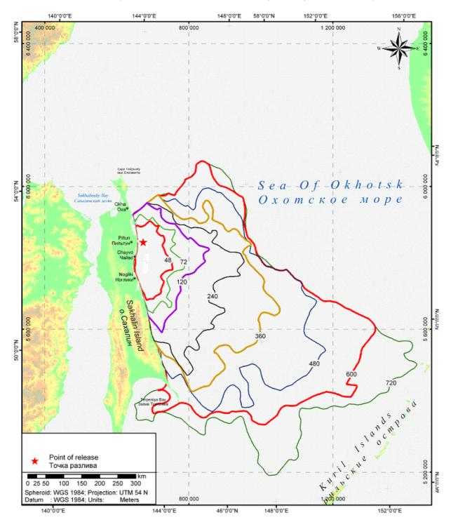
*Figure 2.2 Excursion Envelopes (Risk Zones) for Oil Spills from Piltun-A Platform (Molikpaq): Autumn* (Scenario: Volume: 96m<sup>3</sup>; Cause: Pipeline rupture, REA 2004)
