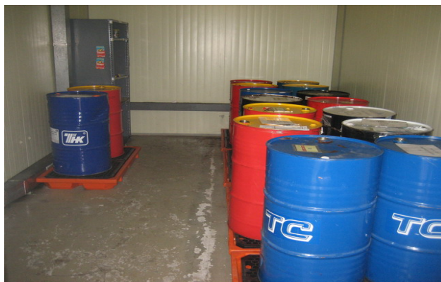
Photo 16 Oil and Chemical storage on gridded drip trays at Sovietskoye PMD
