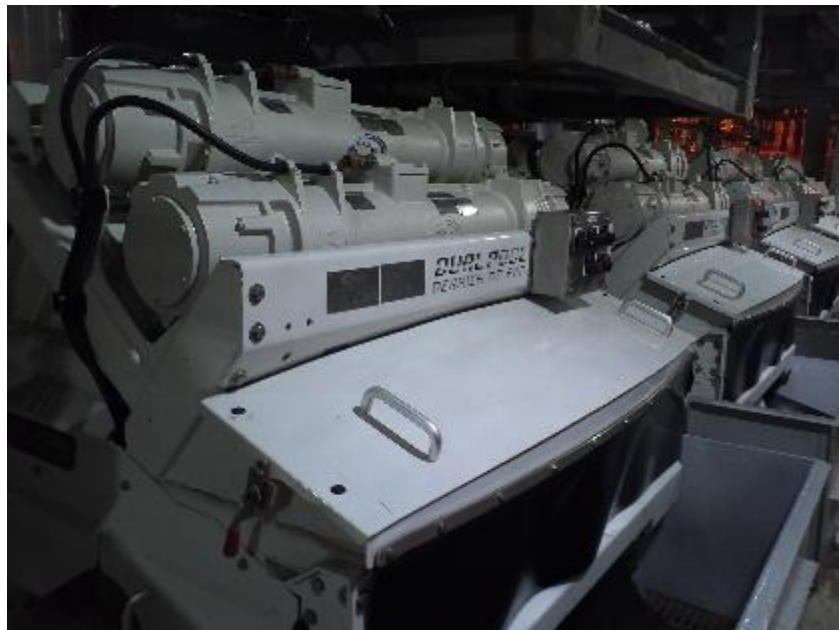
Photo 10. New shale shakers (not yet in operation)
