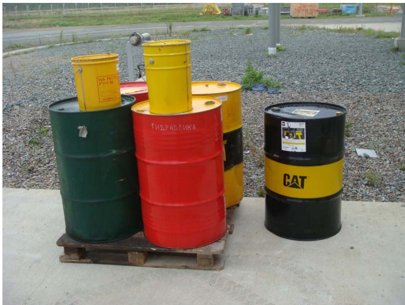
Photo 12: Unbanded, unlabelled drums of unknown liquids outside C107
