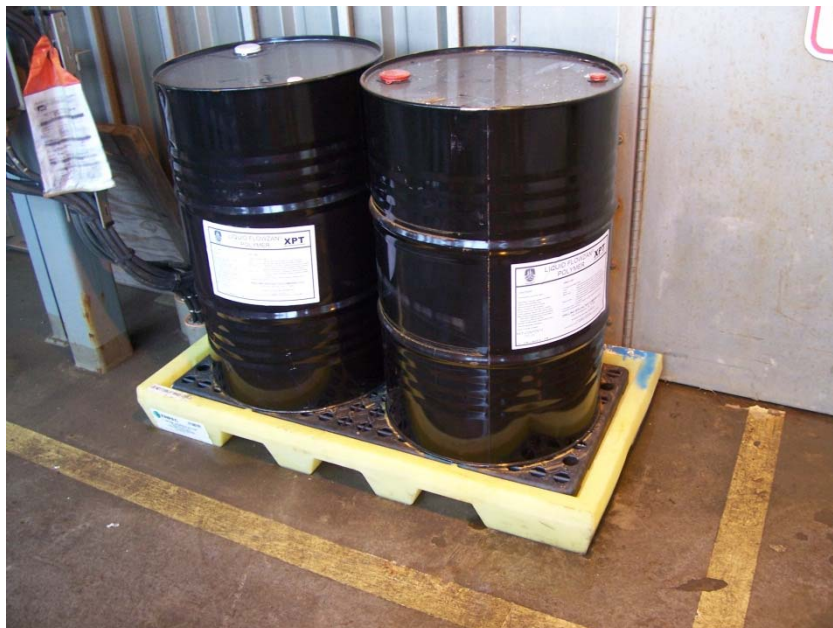
Photo 14: 220 litre drums on 83 litre drip trays
