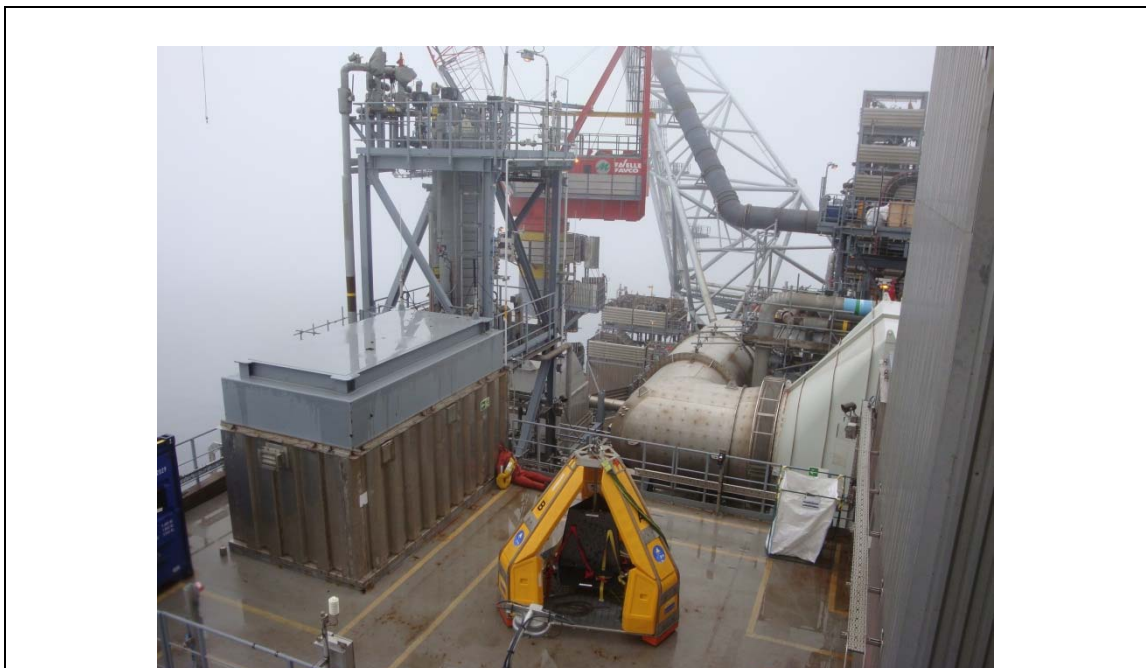
Photo 24: 'Frog' for ship to Platform transfer of personnel
