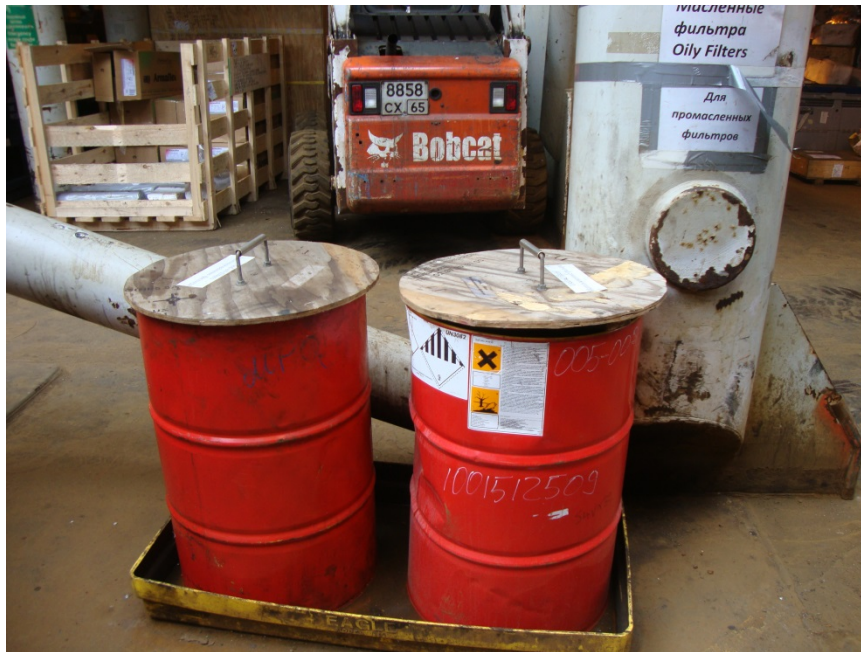
Photo 7. Waste oil filters stored within steel drums
