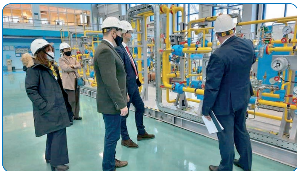
Training is organised at the operating units that simulate gas pipeline sections and block valve stations, are equipped with teleautomatics, and can be controlled from the control unit. It allows not only to master personal professional skills, but also teamwork skills, when the trainees of different pipeline sections are engaged in a single process
