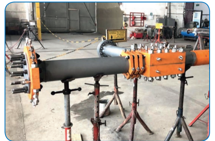
Installation of INTRA SEAL clamps and INTRACOMPOSITE banding on the pipe assembly for testing
