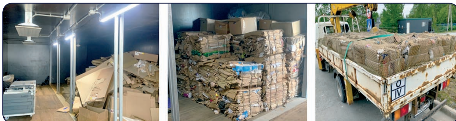
The complex is equipped with a section for paper and cardboard processing and pressing with an industrial press. It helps to increase the weight of one waste batch to be transported 3.5-fold to cut transport costs.
