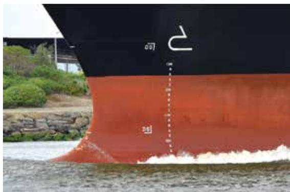
The draft mark scale showing the current draft of the vessel
