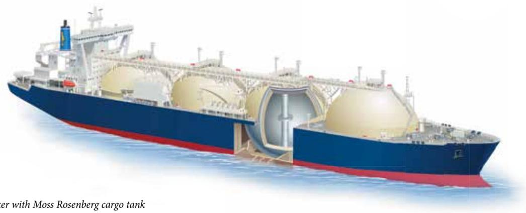
LNG tanker with Moss Rosenberg cargo tank
