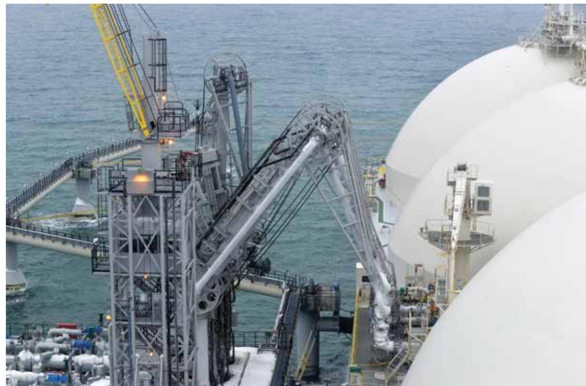
Tanker loading with a marine loading arm, Prigorodnoye production complex, Sakhalin-2 project
